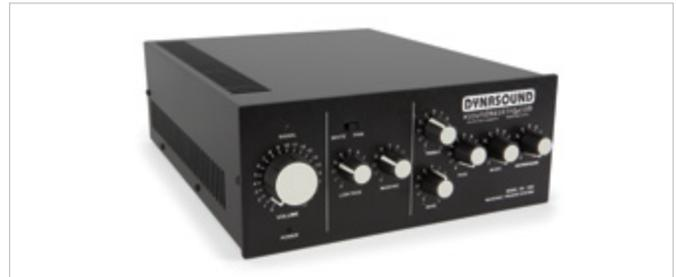
A digital masking generator with adjustable low pass filter for tuning. Incorporates a mixer to introduce paging and music signals into the system. A 40 watt amplifier provides power for up to 40 speakers, or approximately 10,000 square feet (929 m<sup>2</sup>).
